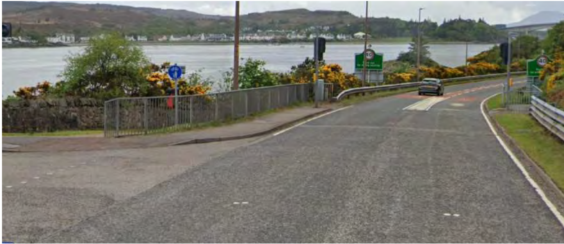
Photo 9E: The traffic light-controlled junction at the Co-op also has a pedestrian phase on demand. The shared footway and cycle route becomes semi-detached here, running behind the railing barrier in the photo. There is a cycle route sign indicating that it is mandatory for cyclists and shared with pedestrians, but this is often ignored or overlooked by cyclists. The footway becomes more closely aligned to the carriageway across the viaducts. There are opportunities to reinforce the mandatory nature of the cycle route at several points west of Kyle.
