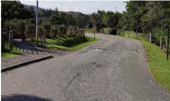
Photo AA: (8.7km) On the approach to the railway bridge and High school the C1221 has a 20-mph limit and raised surface to achieve traffic calming. It also has a strip of green tarmac, but this is not explained to road users and has lost all road paint. The route through Burnside emerges here (on left of photo)
